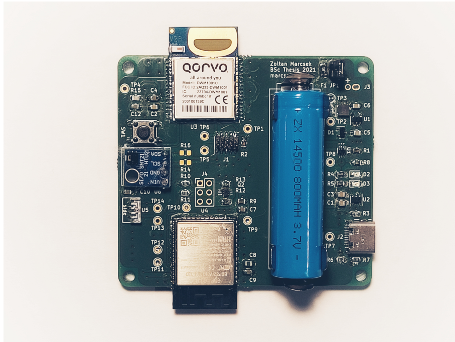
Figure 4.9: The finished, assembled tag with a 14500 lithium battery
